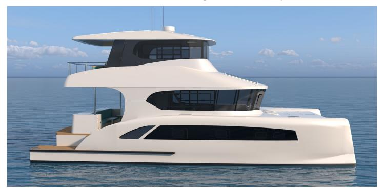
The A044 Pacifica is the first in the AsOne Yachts Ocean series of long-range cruising vessels. Featuring narrow, high efficiency, full displacement hulls, she can cruise for almost 3000nm at 10 knots and sprint at speeds up to 20 knots, with only 180hp engines each side. 800mm bridge deck clearance at full load displacement ensures comfort and performance in challenging sea states.
