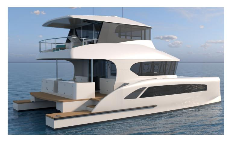
Construction is infused, advanced composite with gelcoat finish, utilising multi-axial fabrics over PVC cores of varying densities. Vinyl ester resin is used throughout the hull and deck construction, with minor items infused or hand laid with polyester resin.
